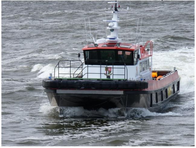
Built at Buckie shipyard and launched in April 2012 The Dalby Derwent is a 17 meter Southboat Catamaran designed to be as flexible as possible. The Derwent can carry 12 passengers and 2 crew. She can carry 8 tons of cargo on her large fore and aft decks. This couple with a top speed of 27 knots make her ideal for the Offshore Renewables Industry.
